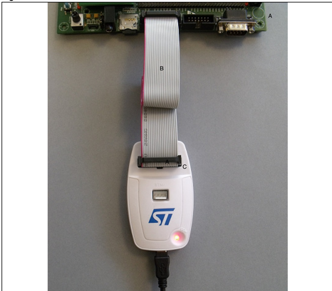
Figure 7. JTAG and SWD connection
